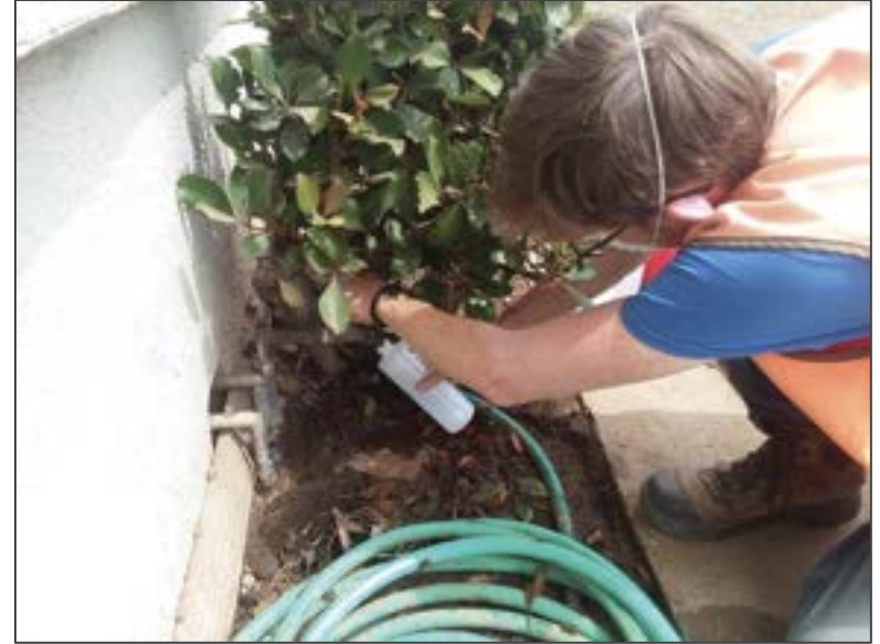
Sample Collection from Nearest-to-Well Hose Bib. Photo by Weber Hayes and Associates.
